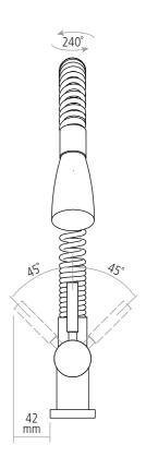
Worktop cut-out 35mm required Note: Pull-out hose extended by 410mm
