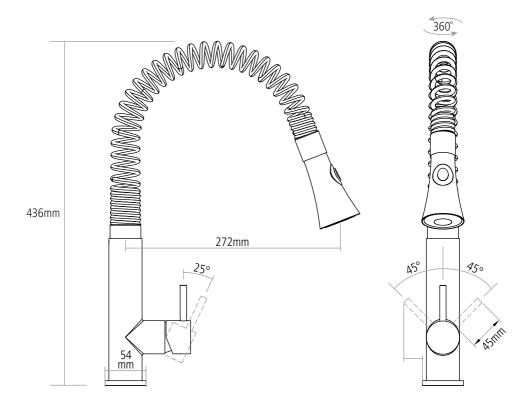
Worktop cut-out 35mm required Note: Pull-out hose extended by 600m
